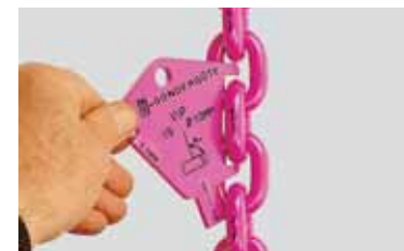
Testing for pitch elongation caused by overload.
